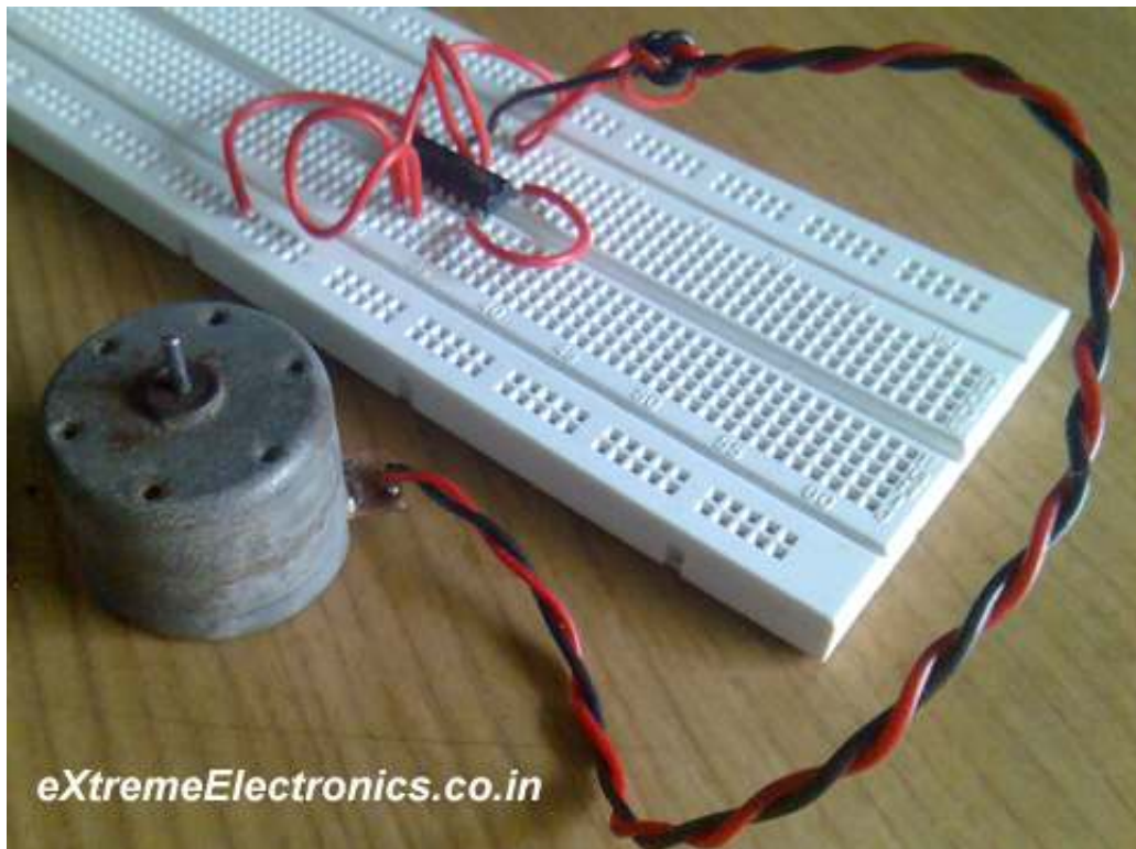
A motor Connected to l293d chip.
